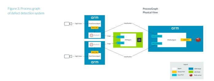
All the agents run in Docker containers. Each node capturing images from the cameras run two containers, one for the camera agent, and one running Redis. Similarly, the node running classification agents runs two containers, one for front image classification, and one for the back.
