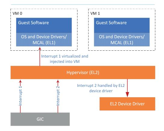
Since all interrupts are initially handled by the hypervisor, the hypervisor can decide if an interrupt should be handled by the hypervisor itself, by an EL2 device driver, or should be virtualized and injected into to a VM. This allows interrupt driven shared/virtual peripherals to be handled. EL2 device drivers can also inject virtual interrupts into VMs if needed.
