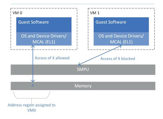
An advantage of using SMPUs, rather than just core MPUs, is that it allows us to create VMs that include not just Cortex-R52+ cores but also other DMA capable components that may be in the microcontroller and are connected to the same memory bus. For example, microcontrollers may include clusters of Cortex-R52+ cores and some special purpose Cortex-M cores.
