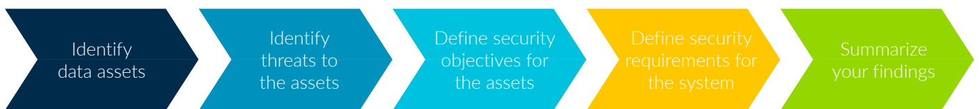
Figure 2 – The threat-based security analysis walks through the steps necessary to identify the data assets in the system, the threat types that those assets will face in the field, how to define the systems security objectives, and finally, how to generate requirements from those objectives that will protect the system’s assets.
